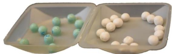
**Impregnated (left) and bare (right) alumina particles**
