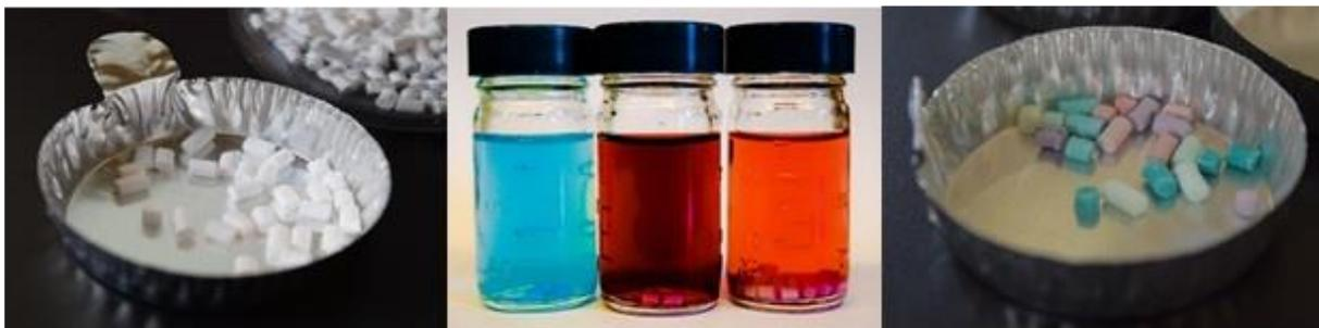
**Figure B3: L-R: Porous alumina supports before impregnation, during impregnation and after impregnation followed by drying at 80°C.**
