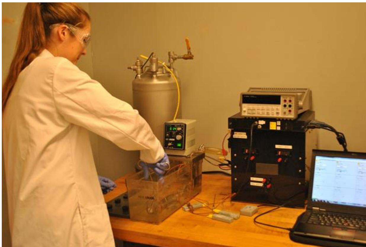
**Measuring the thermal properties of powders in a water bath**
