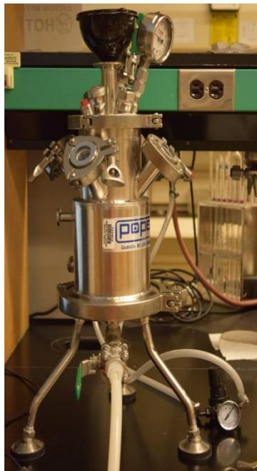
**Figure E1: Benchtop Nutsche filter purchased from Pope Scientific. The vessel has a 1 liter capacity with a 4 inch diameter.**
