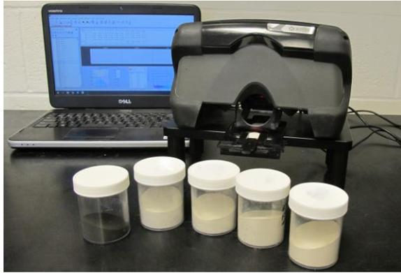
**Figure C2: Colorimeter to analyze concentration of tracer particles.**
