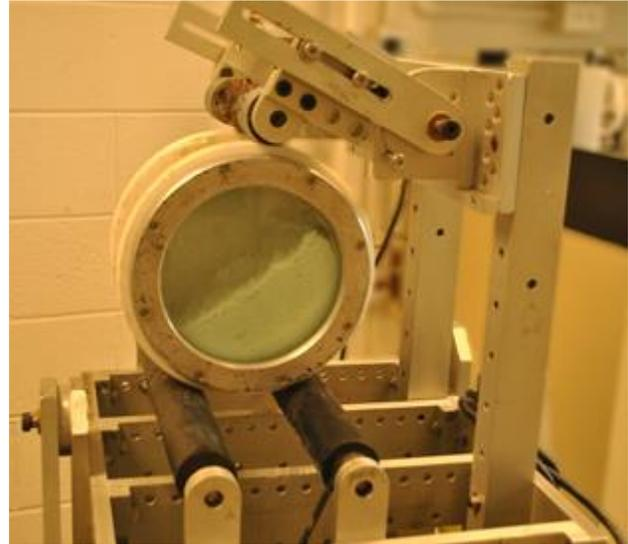
*Alumina powder in a rotating drum*
