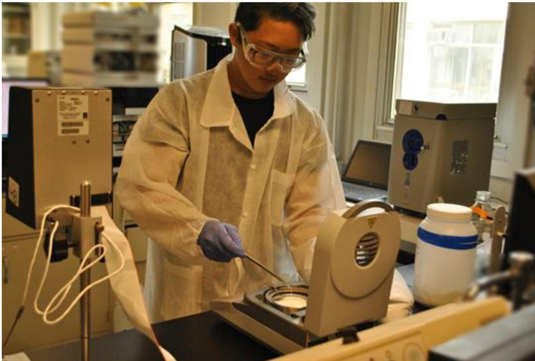
*Measuring the moisture content of alumina powder using a moisture balance*
