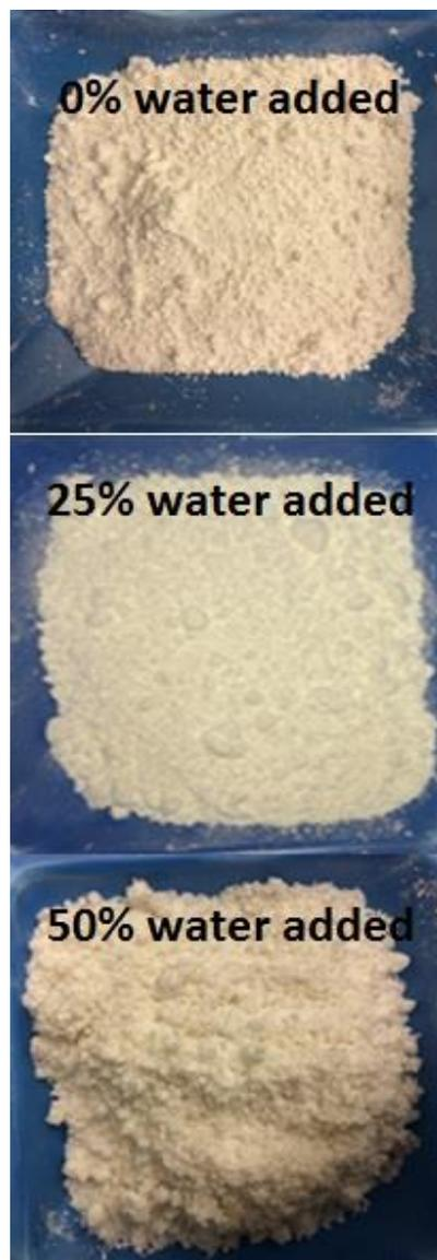
**Figure D1: Alumina powders with different water content.**
